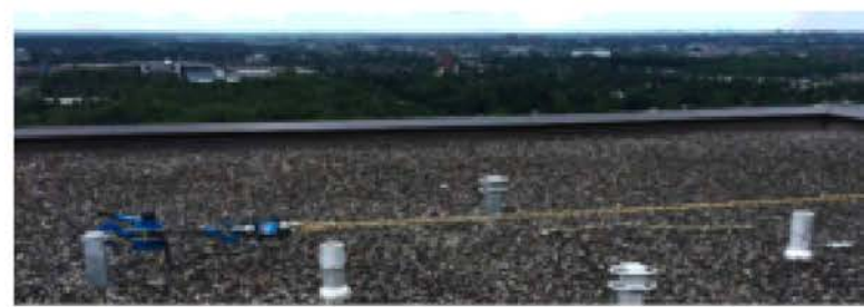
Figure 5. Typical loading apparatus between pedestal anchors
